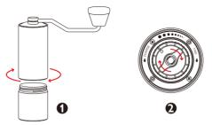
Pull out the container. Set up coarseness by turning the scale at the bottom of the body.
