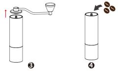
Fasten Body with the container. Then open the lid and pour coffee beans inside from the top of the grinder (less than 20q).
